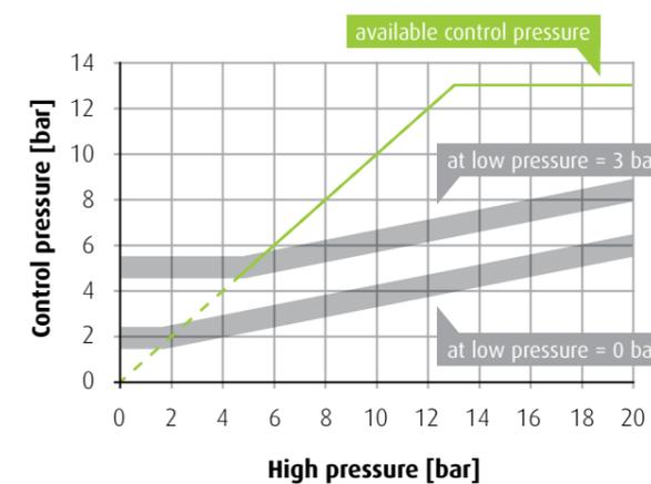
Characteristic curve of the cooling oil valve: control pressure required for opening the valve in dependency of the pump pressure.
